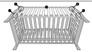
8. Remove any bedding and mattress from the cot. Loosen all bolts by 2 or 3 turns, this will help when removing the sides and moving the base up or down. Carefully turn the cot on it's back so that the front cot side (C) is uppermost. Fully undo the 4 bolts (i),(ii),(iii),(iv) and remove the front cot side (C). Put the cot side (C) and the 4 bolts safely to one side.
