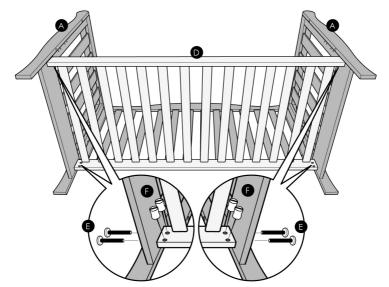
3. With the cot still on its side, carefully place the cot base (D) in between the two cot ends (A) at your desired height. Fix the cot base (D) to the cot ends (A) using 8 bolts (E) and 8 barrel nuts (F) tighten with Allen key (G).
