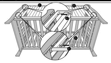
11. Attach the front cot side (C) by lining up the holes on the cot side with those on the edge of the cot ends. Insert 4 bolts (E) through the holes in the cot side and tighten into the cot end using Allen key (G).
