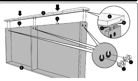
5. With the partly assembled drawer still on to its back panel (B), place the drawer front panel (A) onto the partly assembled drawer so that all the cam lock screws (H) and wooden dowels (J) fit into their corresponding holes.
