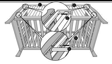
4. Attach the front cot side (C) by lining up the holes on the cot side with those on the edge of the cot ends. Insert 4 bolts (E) through the holes in the cot side and tighten into the cot end using Allen key (G).
