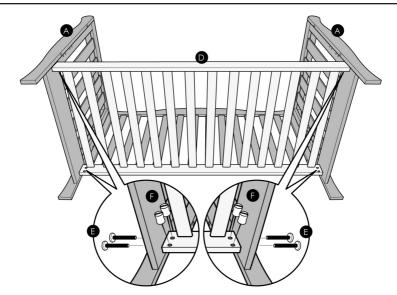
10. Reposition the cot base (D) in between the two cot ends (A) at your desired height. Fix the cot base (D) to the cot ends (A) using 8 bolts (E) and 8 barrel nuts (F) tighten with the Allen key (G).
