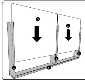
3. Carefully turn the partly assembled drawer on to its back panel (B) as shown. Slide the base panels (G) along the slots in the side panels (C), (D) and centre partition (E) and into the slot on the back panel (B).
