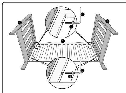
2. Take one cot end (A) and line up the holes on the cot side with those on the edge of the cot end. Insert 2 bolts (E) through the holes in the cot side and tighten using Allen key (G). Attach the second cot end (A) in the same way.
