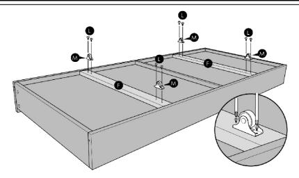
6. Turn the drawer face-down, line up the wheels with the pilot holes on the base supports (F) and using a cross head screw driver attach two wheels (M) to each base support (F) using screws (L).
