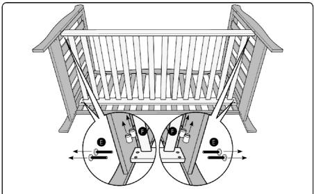
9. Undo and remove all 8 bolts (E) and barrel nuts (F) that hold the base in place.
