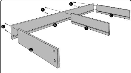
2. Attach the left side panel (C), right side panel (D) and centre partition (E) to the back panel (B) using 6 wood screws (K) and tighten using a cross head screwdriver.
