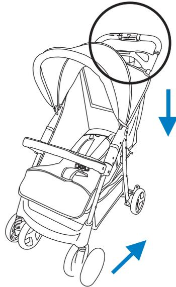
Push frame together and lock the lock hook.
