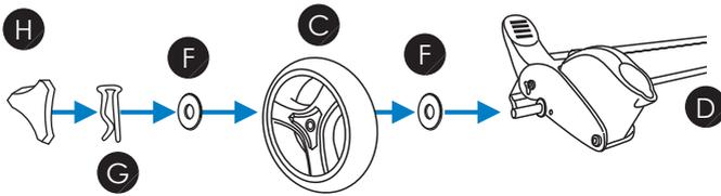
Attach the rear wheel axle (D) to the rear of the chassis. Push to the rear of the chassis. Push in until you hear a "click".
