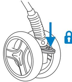
To go back to 360° swivel mode, push lever upwards.
