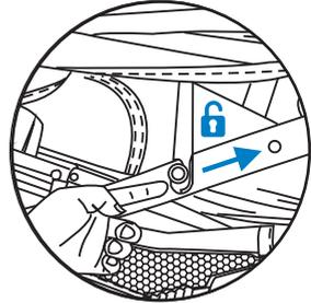
Lift the handle upwards, at the same time the front legs will move forwards. Lift the frame until it is completely open, you will hear a "click" indicating it is locked into place.
