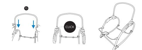
**6.6.** Fit the top of the seat pad (I) onto the rear connector tube (G). Next fit the lower part of the seat pad onto the music box connector tube (F).
