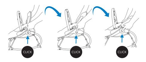
**7.2.** To switch to a rocking mode lift the kickstand (D) under the rocker. To switch into a stationary mode, push the kickstand out to prevent rocking.
