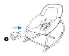
**6.9.** Insert the toy bar into the sides of the rocker, please notice both clips should "click" when in place.
