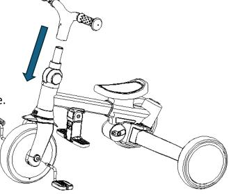
3. Unfold the Seat (C) and then fix onto the seat of the Chassis (A) as shown left, until it clicks into place. Pull the Seat (C) from side to side to ensure that it is securely in place.
