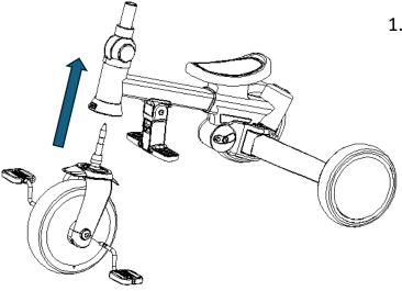
1. Insert the Front Wheel (D) into the Chassis (A) as shown in the diagram left.
