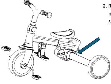
9. Repeat the above steps 6 & 7, then remove the metal connecting rod from the Chassis (A) as shown left.
