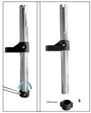
31. Loosen the seat adjustment knob (J) on the underside of the seat unit (I).
