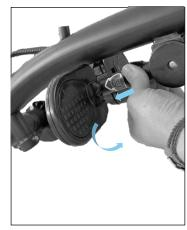
14. Rotate the steering rod (G) backwards until it is horizontal
