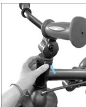
8. To fold the handlebar, push the circular button
