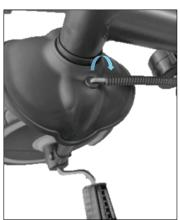
15. Insert the back of the steering rod into the hole on the arm of the steering post (F) and secure with the nut provided. Use the spanner to tighten (M)
