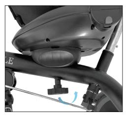
10. Insert the steering post (F) into the tube at the back of the trike frame (B)
