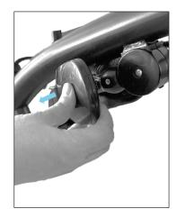
13. Insert the front of the steering rod (G) vertically into the hole in mudguard (D)
