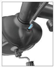
30. Pull the collar down on the footrest tubing to release and rotate downwards. Reverse the process to fold the footrest
