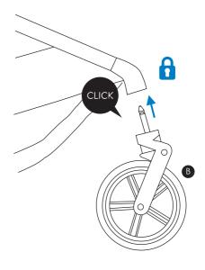
**To remove** the front wheels, simply press the button at the back of the wheel socket and pull down.
