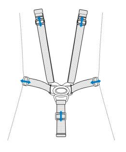
There are 2 shoulder height positions. Undo the harness and remove the shoulder pads. Thread the end of the harness through the slots at the front of the backrest to adjust the height position.
