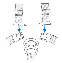
Insert the completed buckle into the buckle housing until it engages securely in place. Listen for the "click".
