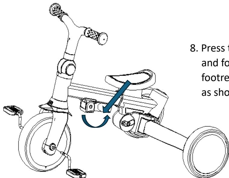
8. Press the button on the footrest and pull down and fold towards the rear wheels folding the footrests inwards and it should click into place as shown left.
