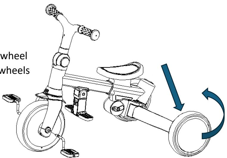
10. Press the buttons on the inside of the rear wheel frame on the Chassis (A) and fold the rear wheels inwards.
