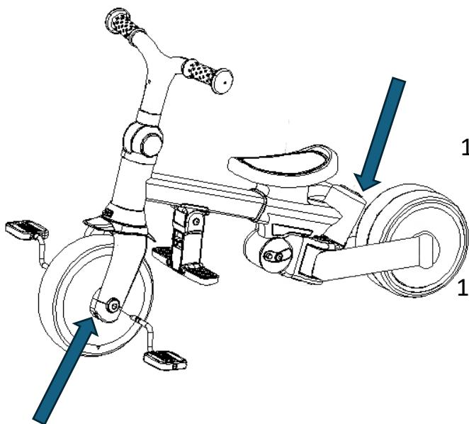
11. Press and hold the button on rear of the Chassis (A) as shown left and then fold the rear wheel frame on the Chassis (A) inwards until it clicks into place as shown left.
