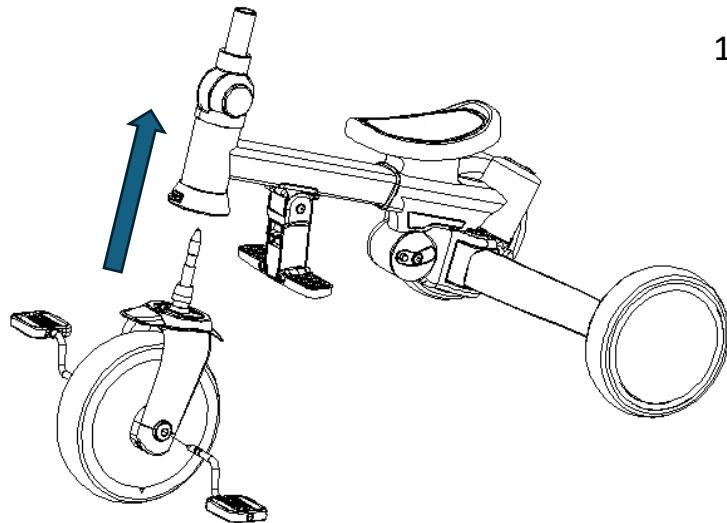
1. Insert the Front Wheel (D) into the Chassis (A) as shown in the diagram left.
