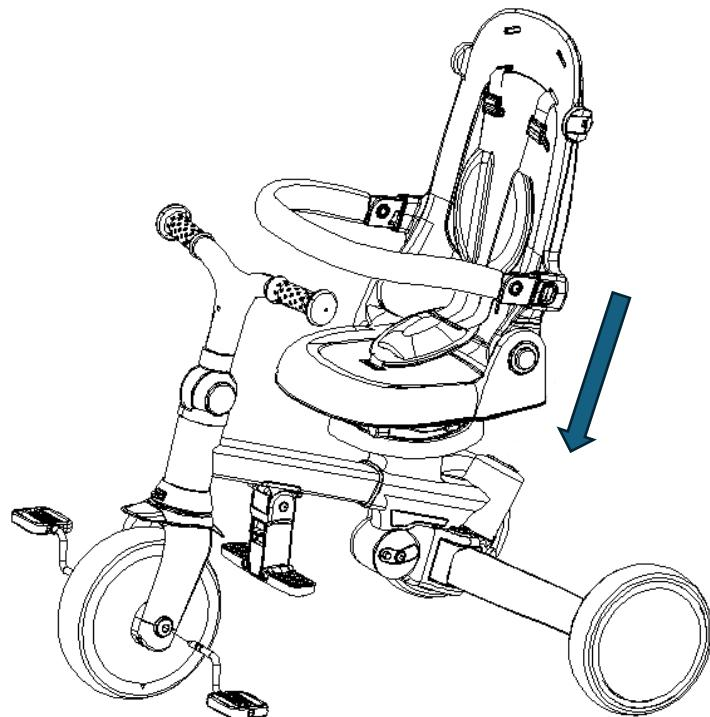
Note: The backrest can be adjusted by pulling on the handle at the rear of the Seat (C) and adjusting the position of the backrest accordingly, the backrest will click into place.
