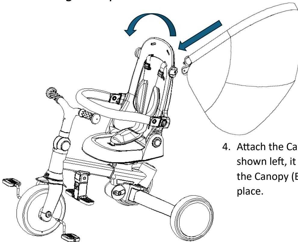
4. Attach the Canopy (E) to the Seat (C) as shown left, it will click into place. Pull on the Canopy (E) to ensure it is securely in place.
