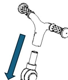
2. Insert the Handlebar (B) onto the Chassis (A) until it clicks into place. Pull up on the Handlebar (B) to ensure it is securely in place.
