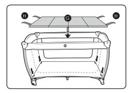
5. Place mattress (G), padded side up, into the travel cot. Thread straps (H) through the four slots on the base and attach them to the velcro fasteners on the underside of the travel cot.
