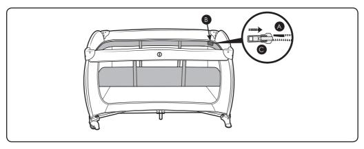
1. Locate zip attachment (A) under fabric flap (B) on one corner of the cot. Attach the zip slider (C) on the bassinette to the zip insertion pin and fasten the zipper until the bassinette is attached. Conceal the zip slider with the fabric flap (B).
