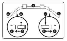
2. Connect all tubes, inserting the narrow end of tube (B) into the wider opening of tube (A), as shown, press in spring pin (iii) and push the tubes together until the spring pin locks into place.
