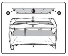
3. Place mattress (G), padded side up, into the travel cot, so that the four velcro tabs on the underside of the mattress connect to the four tabs on the bassinette base.
