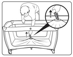
3. Grasp the webbing handle in the centre of the cot base and pull upwards fully.
