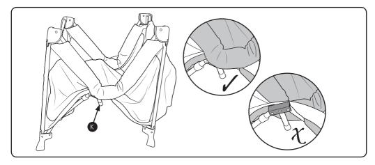
7. With all four rails unlocked, ensure that the central leg (K) is contained within the sides of the  $\cot$  and not on the outside.
