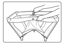
4. With the centre of the cot base pulled up, balance the cot by keeping hold of one corner before moving to the next step.
