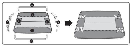
1. Feed the two side tubes (A) through sleeves (i) and end tubes (B) through sleeves (ii).
