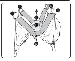
2. Spread the top corners (i, ii, ii, iv) part way out, ensuring the centre section (C) remains in the raised upright position. Lift side rails (D) to the 'lock up' position and repeat with the end rails.
