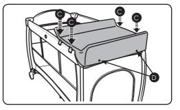
3. Attach the four hooks (C) on the underside of the changer to the cot sides, pull the flap of fabric over the cot end and fasten press studs (D) to the cot end.
