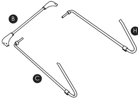
**6.2.** Lift the flip clip on both sides of the rear connector tube and lift the left support frame and right support frame into the rear frame tube. Close the flip clip over the tube and press down until the flip clips lock in place.
