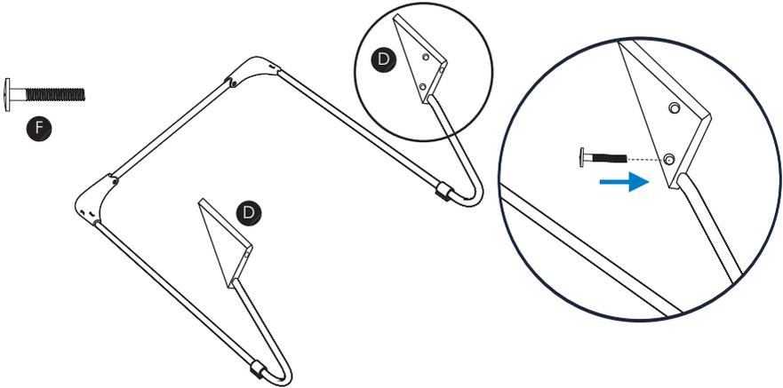
**6.4.** Fit both ends of the footrest frame (G) to the plastic connectors and secure with screws (D). Ensure the recess for the vibration box is level.
