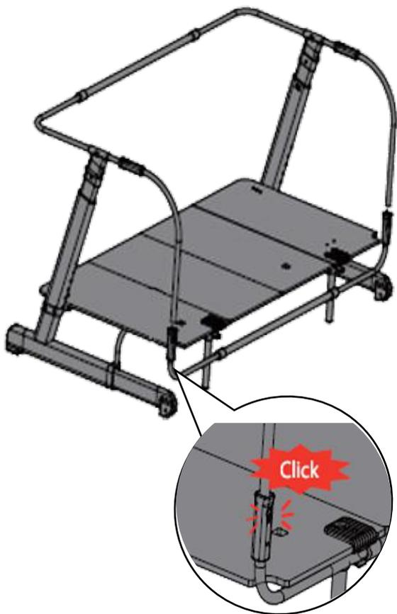
24. Attach the Short Top Railing (G) to the Support Feet (J), simply slot the bar into the corresponding brackets on the Support Feet (J). The bar will click into place when secure, as shown right.
