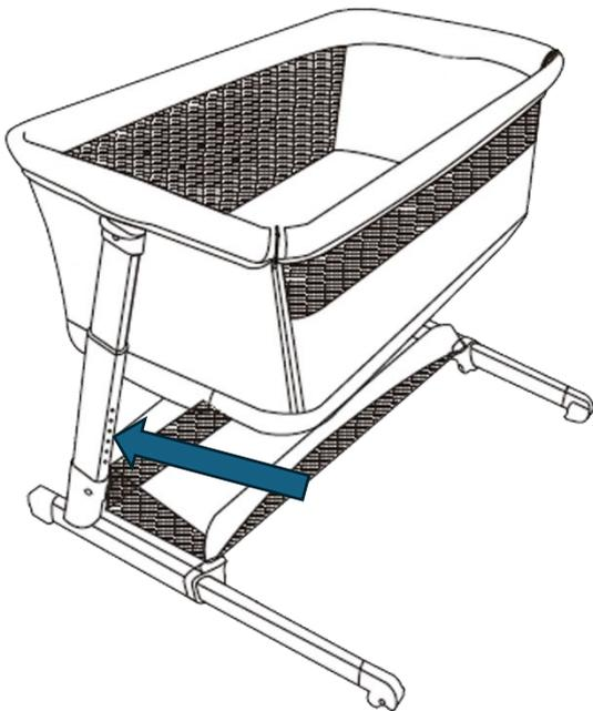
5. To adjust the crib position, simply press the spring pins either side and lower or raise the Crib Body (A). The crib will click into place and the spring pin will protrude through the frame.
