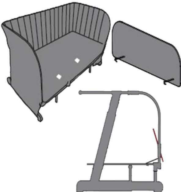
28. Attach the Guardrail (L) to the Toddler Bed Body (C) and Base Board (P) using the 'L shaped' metal bar at the rear of the Guardrail (L) as shown left.
