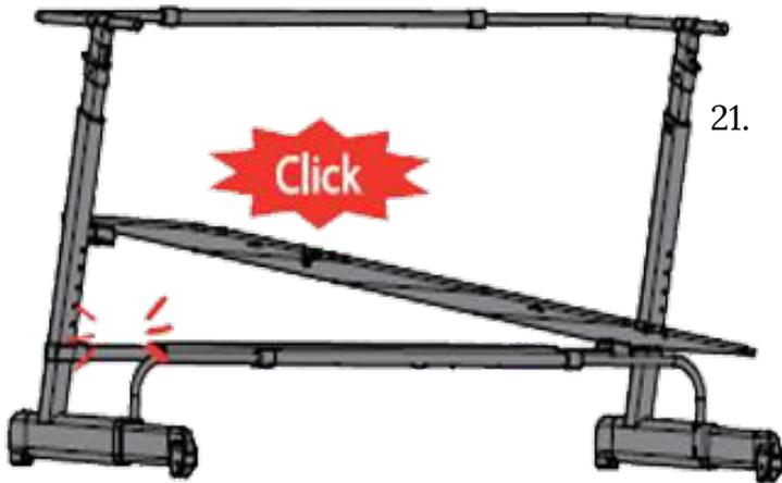
21. Attach the Base Board (P) onto the Rear Support Bar (H) as shown left. The board will click into place when secure, as shown left.
