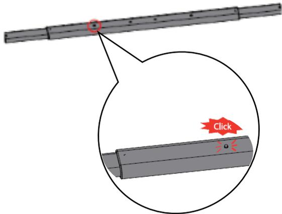
15. Extend the Rear Support Bar (H). To extend press the springs pins in on either side and pull the telescopic part out. The bar will click into place when secure, as shown left.
