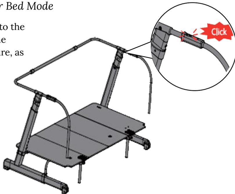
24. Attach the Short Top Railing (G) to both of the Lateral Support (K) as shown left. The bar will click into place when secure, as shown left.
