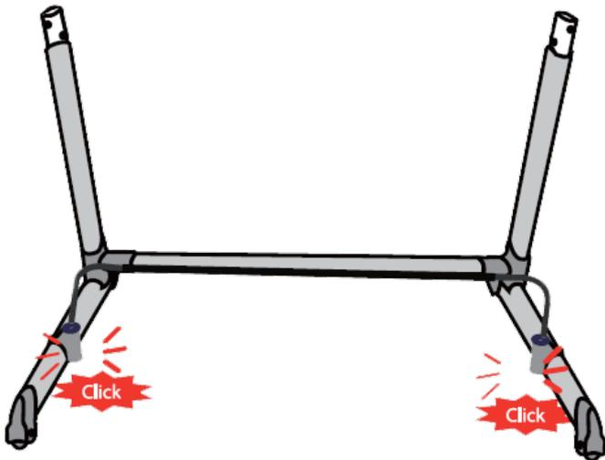
2. Insert the Front Brace Bar (I) into both of the Side Frames (E) as shown left. When fully inserted the Front Brace Bar (I) should click into place and the spring pin will pop out of the corresponding holes on the Side Frames (E).
