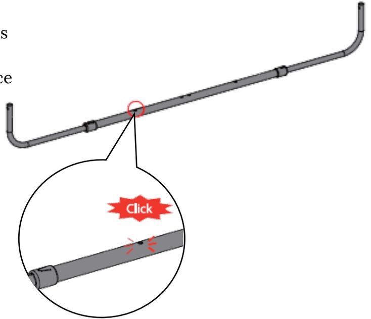
18. Insert the Front Brace Bar (I) into both Side Frames (E) as shown left. The bar will click into place when secure, as shown left.
