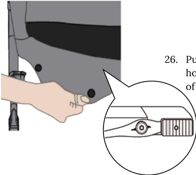
26. Pull the side flaps of the Toddler Bed Body (C) down and hook the holes over the corresponding buttons on the base of the Side Frames (E).
