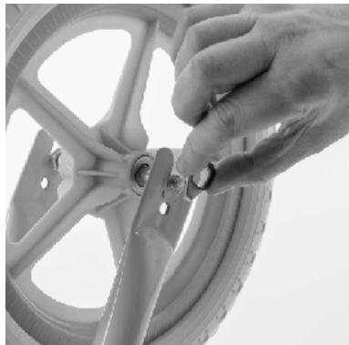
5. Slide the wheel axle (H) into the wheel fork. The sleeve and nut should be on the inside of the fork.
