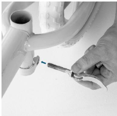
9. Insert the seat unit (E) into the bike frame (A) when it is at the desired height, push the seat adjuster clamp (F) forward until it completely closes. The bar must be inserted until the minimum depth markings are hidden.
