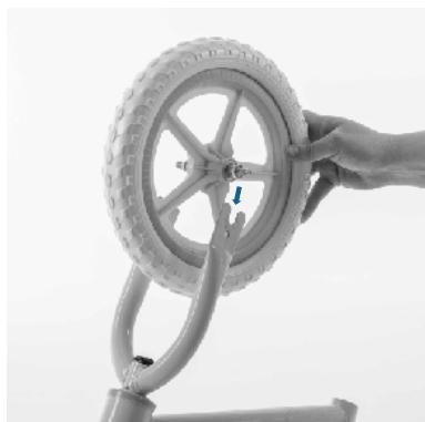
6. Use the spanner (J) to tighten the domed locking nuts equally on each side of the bike, until the wheel forks are pulled together and there is no axle rod visible.
